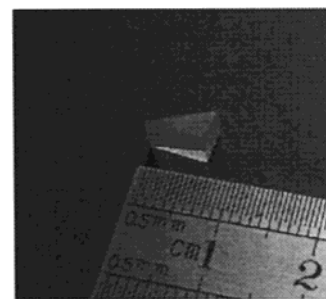
Figure 4. ZBP prism (6.4 × 3.6 × 4.2 mm).
